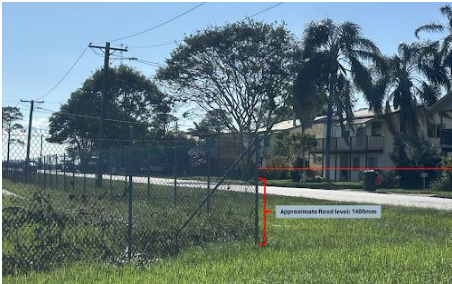
Figure 6. Rawson Street at Smithtown showing abandoned homes and approximate flood height of 1400 mm (red line) determined from football field fence debris and flood water lines on homes
