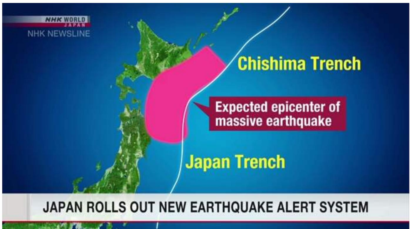
Figure 1. Expected rupture zone (shown in pink; “epicenter” should say “rupture zone”) of the large earthquake for which alerts will be given by JMA. Source: NHK News.
