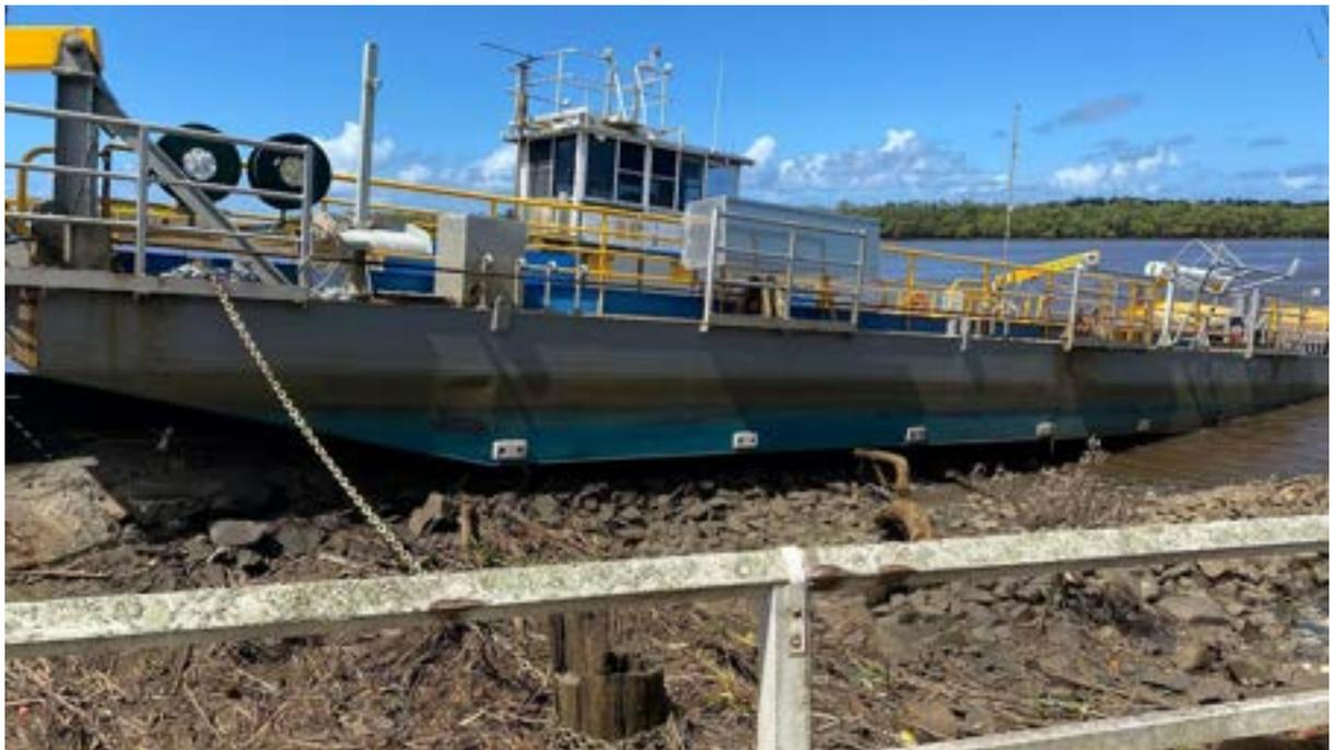
Figure 12: The Burns Point Ferry, stranded after its submarine cable snapped during the flood. Note the chain mooring the ferry to the piling on shore in the foreground, which prevented the total loss of the vessel
