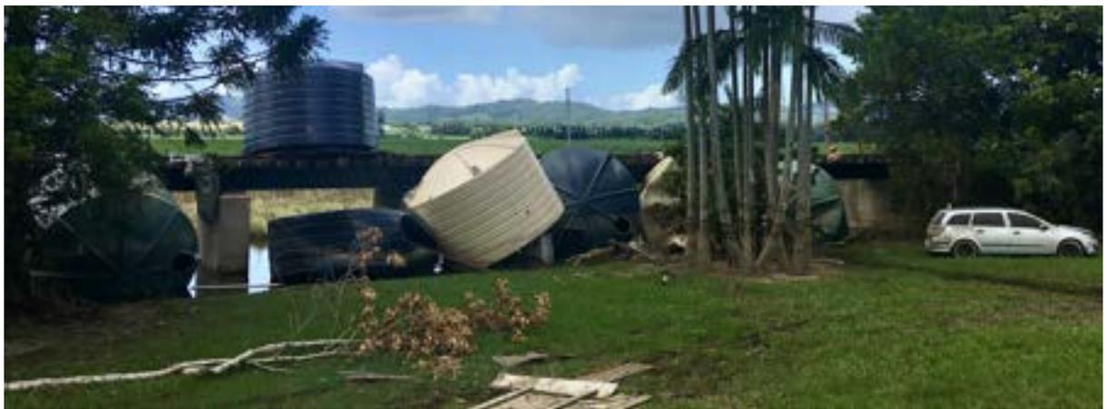
Figure 14: Plastic water tanks are easily transported by flood waters as seen in this example from South Murwillumbah where a number have been forced beneath a railway bridge.
