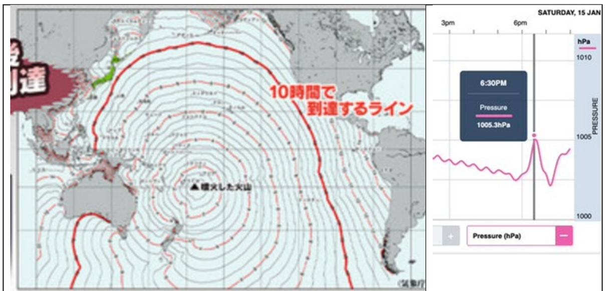
**Figure 1.** Left: Predicted tsunami travel times throughout the Pacific Ocean for an earthquake generated tsunami. The red contours are 2 hours apart and the black contours are 30 minutes apart. Source: Watada (2022). Right: Arrival of the air pressure wave in Sydney at 6 pm. Source: BoM.
