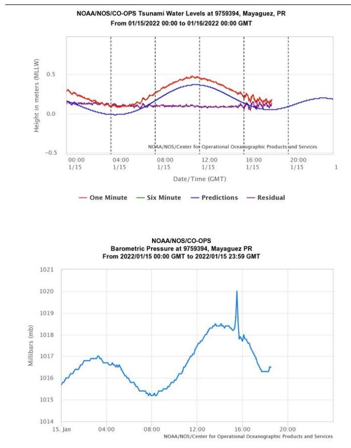
**Figure 3:** Tide gauge (top) and barograph (bottom) of the Tonga explosion at Mayaguez, Puerto Rico. The purple line in the top panel shows the record after removal of the tides. Source: Dr Greg Dusek, NOAA.
