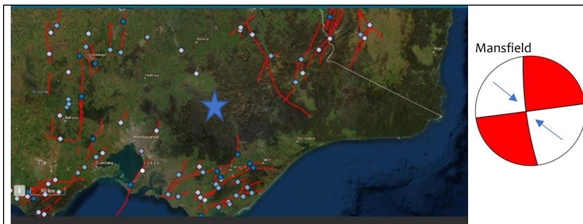
Figure 1. Left: The epicentre of the Mansfield earthquake is shown by the blue star, and identified potentially active faults are shown by red lines. Right: Earthquake focal mechanism in map view showing the orientation of the two possible fault planes; the arrows show the direction of maximum horizontal compression. Source: Geoscience Australia.
