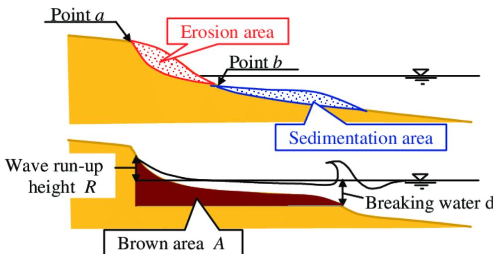
Figure 3. A cross-sectional beach profile showing simplified erosion during a storm event (top panel), and consequential depleted beach and higher water mark post-storm (bottom panel). Source: Yamamoto et al. (2012)
