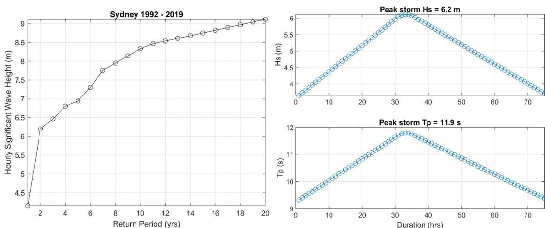
Figure 4. Left panel: return periods associated with wave heights at Sydney. Right panel: synthetic storm curve for the 2-year return period storm for wave height (top) and wave period (bottom).  $H_s$  = significant wave height,  $T_p$  = peak energy wave period. The Sydney wave buoy is maintained and operated by Manly Hydraulics Laboratory (MHL). Wave data are available on request from MHL.
