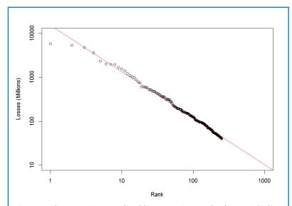
Figure 2: The top 300 normalised losses against rank. The straight line shows a Pareto (power law) distribution.
