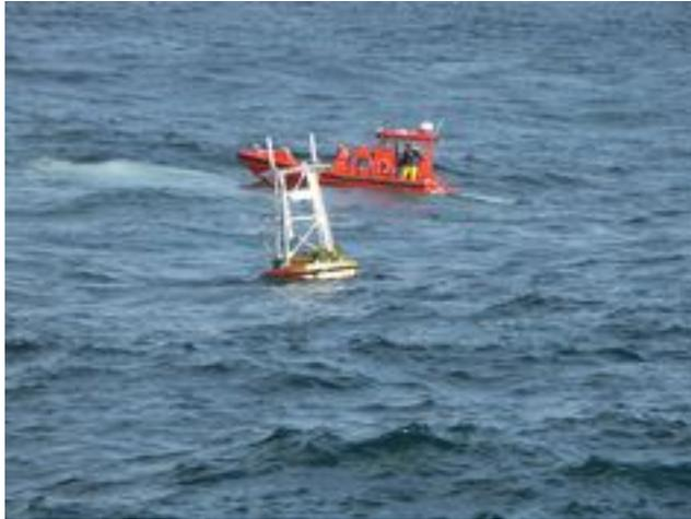
*NOAA tsunami detection buoys can come unmoored in the deep ocean, as this one did, requiring recovery and replacement – and not detecting any usable data until it's back in place.*
