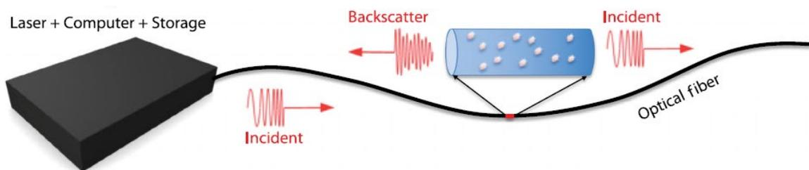
**Figure 1.** Backscattering from defects in the fibre that carries information about the strains in every few metres of the cable. Source: Zhan (2020).
