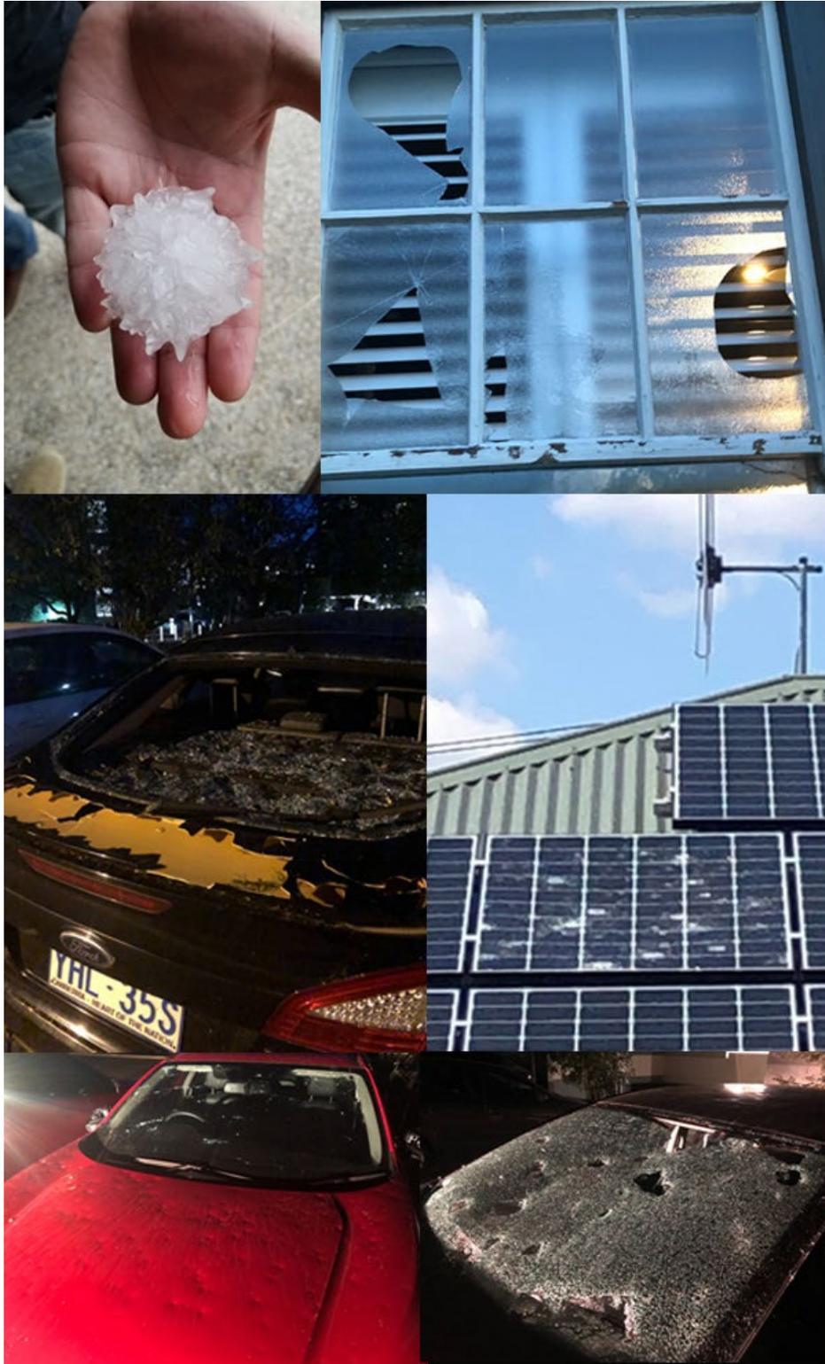
**Figure 1.** Photographs of damaged cars, windows, and solar panels from Barton and Civic Square in Canberra.
