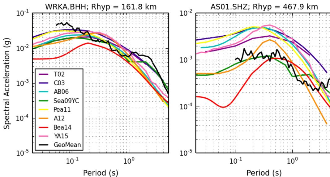
**Figure 2.** Comparison of response spectra of ground motions recorded at two stations (black lines) with the predictions of ground motion models. A12 (Allen et al., 2012; orange lines) and Sea09YC (Somerville et al., 2009; green lines) are the two Australian models; the others are for eastern North America. Source: Trevor Allen, personal communication)
