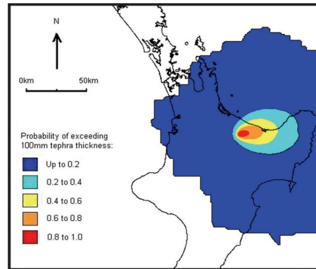
**Figure 1:** Multiple phase tephra fall footprint established using ASHFALL (Hurst, 1994). An erupted volume of 5km<sup>3</sup> is comparable to that erupted throughout the Vesuvius AD 79 or Pinatubo 1991 eruptions and is relatively modest for Okataina volcanic centre.
